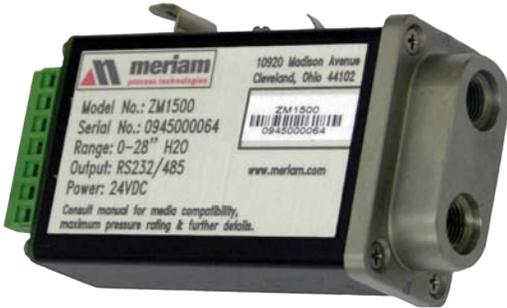
Meriam's compact, M1500 Digital Pressure Transmitters are ideal for pressure measurement needs from 10" H<sub>2</sub>O to 3000 PSI Full Scale. Output options include digital (RS-232, RS-485 and USB) or analog (mA or V DC). Choose from differential (dry/dry or wet/wet), gauge, compound or absolute pressure types – see the table inside for complete details.
