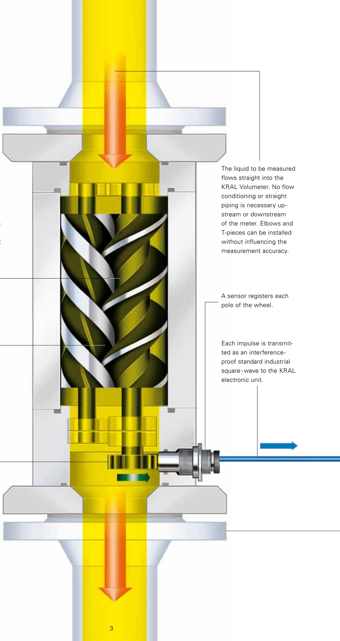
The liquid to be measured flows straight into the KRAL Volumeter. No flow conditioning or straight piping is necessary upstream or downstream of the meter. Elbows and T-pieces can be installed without influencing the measurement accuracy.
