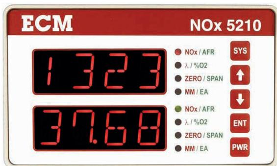
ECM's NOx 5210 is a versatile and highly integratable NOx, Lambda and O2 analyser for the development of engines, combustion systems and after treatment systems. NOx, Lambda and O2 are measured using a ceramic sensor that is mounted in the exhaust of the engine.
