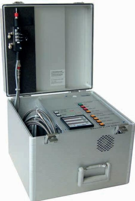
The Tetratec CFO-Sx00 is commonly used for calibration of CVS dilution system or SHED chamber. It uses electronic control to inject a known dose of gas (either propane or carbon monoxide) into the CVS system to check the calibration of the measurement instrumentation.
