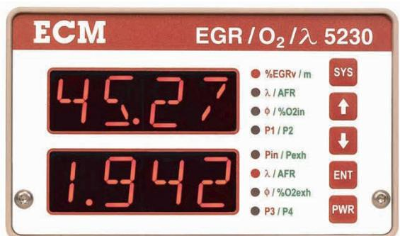
Exhaust gas recirculation (EGR) is a powerful control used to suppress NOx emissions in engines. As important as EGR is to the operation of engines, in the past there has been no simple and compact way to measure it. Now there is with ECM's EGR 5230 Analyzer.
